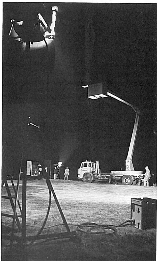
Fig.3 Night photography to record the surface undulations of the turf (Ph. E. Morgan).
