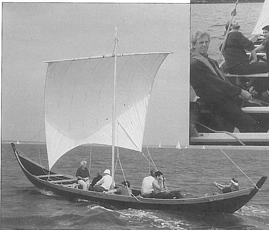
Above: Sæ Wulfing, wind to the fore reaching Force 3 (4–5 knots). The sail is reefed to reduce the load on the stretchy rigging and bending mast! (Photo: Paul Calvert)
