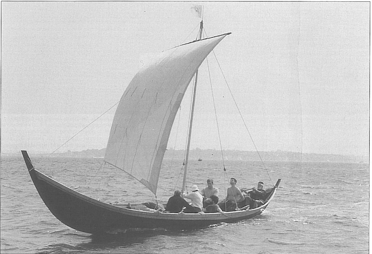
Sæwulfing – a half-scale replica of the ship found in Mound 1 at Sutton Hoo, built by Edwin Gifford and the Saxon Ship Project, here seen under sail on the Solent (Photo: Jim Smith)
