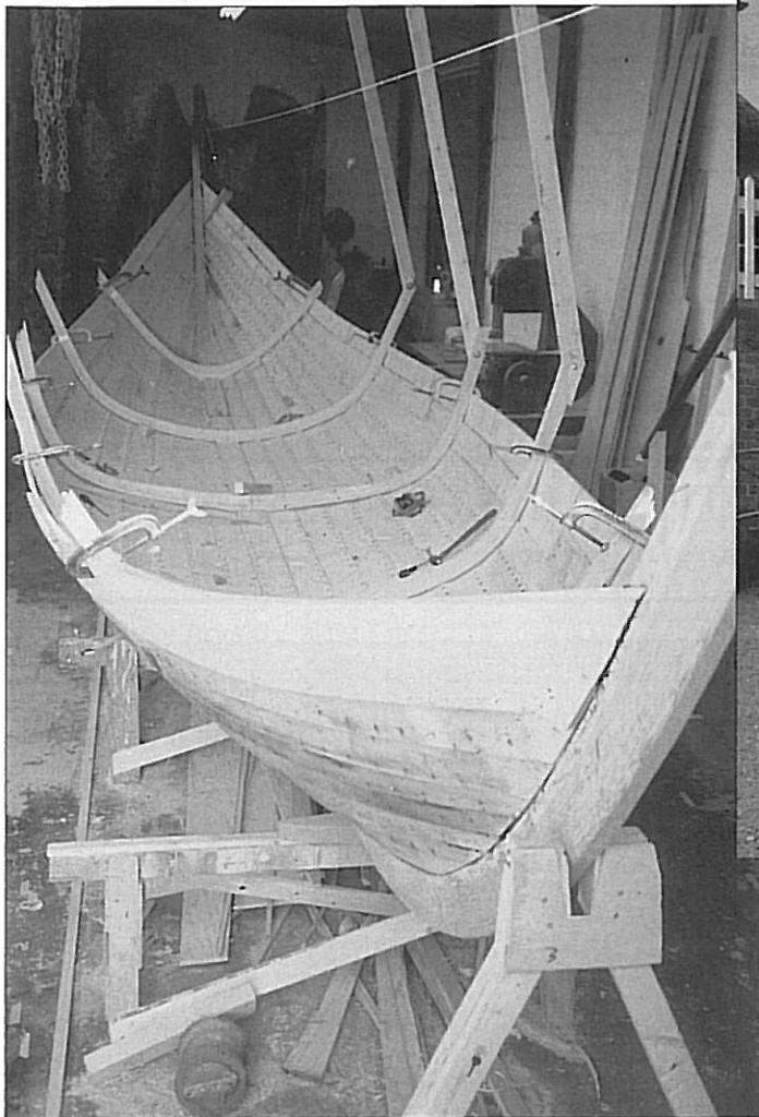
SæWulfing under construction: the planking is complete but not yet fastened to the frames. Note the two upper strakes in oak (Photo: Edwin Gifford)
