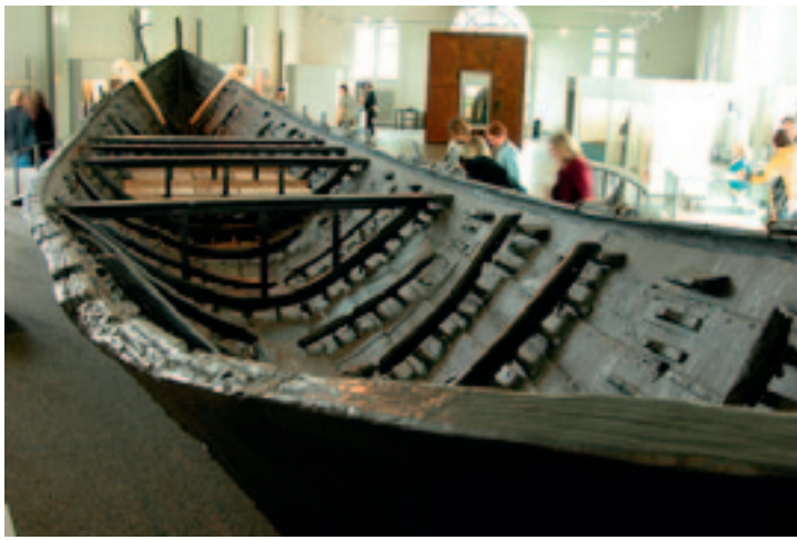
The Nydam ship in Gottorp Castle, Schleswig, Germany. Clinker built of oak, 23m × 3m, it was pulled from a Danish bog in 1863 and has been dendro-dated to c. 310–320. (© Erik Christensen)
