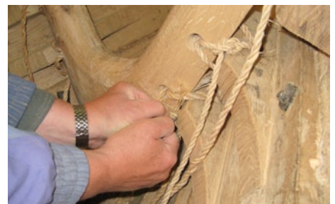
The ribs being tied in to the strakes using twisted lime bast fibres.
