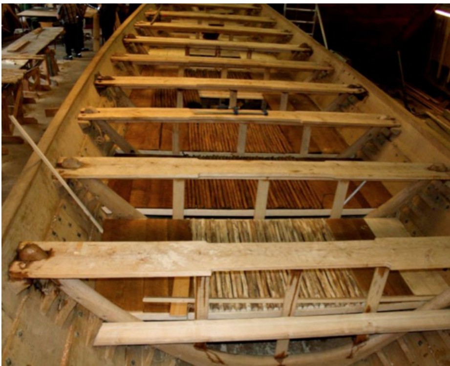
Coming along nicely: the Nydam replica with half the floor fitted
