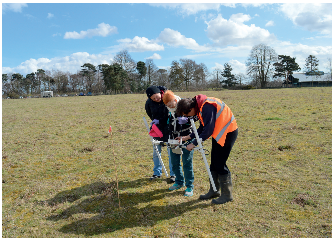
Geophysical surveyor from Suffolk Archaeology teaching fluxgate gradiometer setup to a National Trust volunteer and Sutton Hoo visitor.
