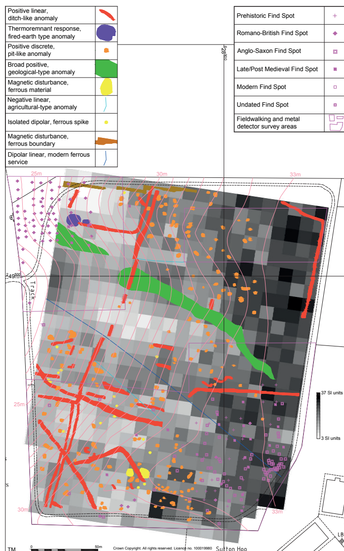
SACIC and Historic England magnetometer data interpretation and find spots by phase, overlying magnetic susceptibility greyscale data.
