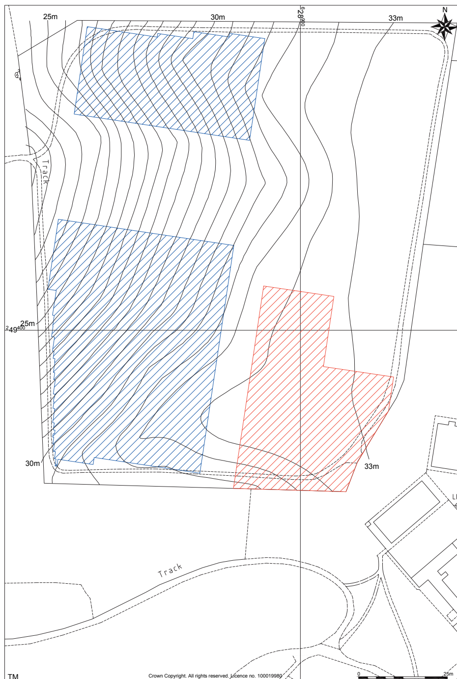
SACIC survey areas, earth resistance meter in red, fluxgate gradiometer in blue, magnetic susceptibility meter undertaken across the whole field.
